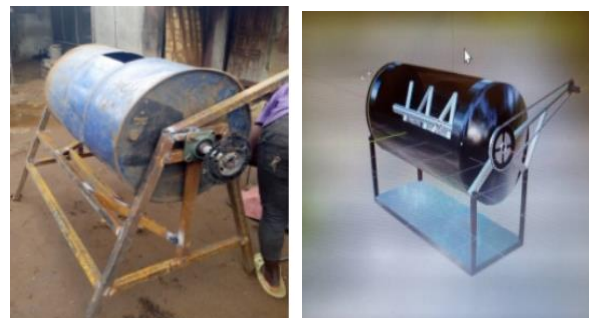
Plate 2. The 250L bioreactor Actual, LEFT and Computer aided design (CAD), RIGHT.
