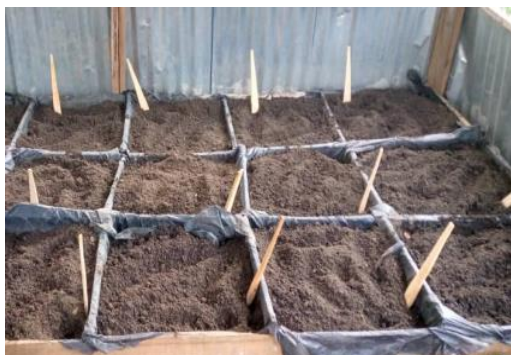
Plate 3. Biocells each 50cm x 50cm and 15cm deep under treatment.
